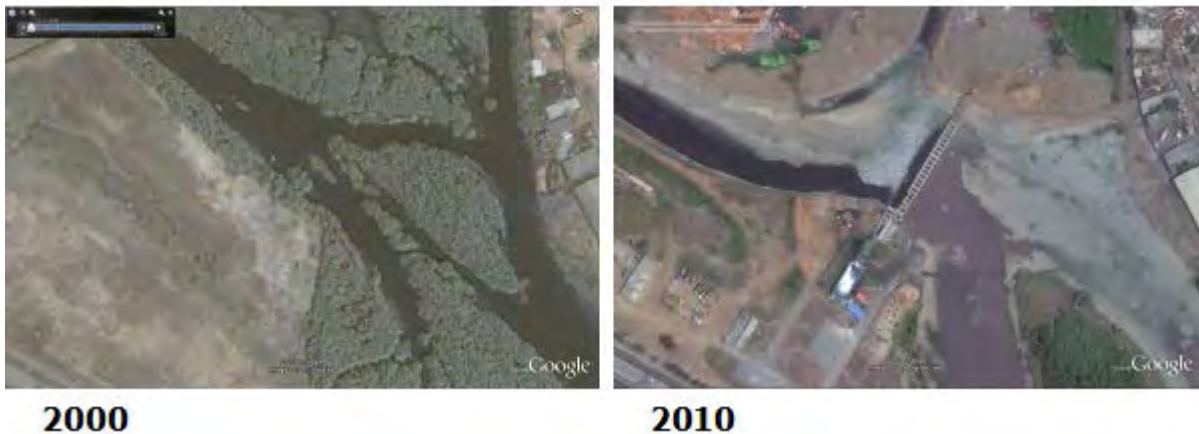
Figure 35. Korle Lagoon – in 2008 just upstream of Korle Lagoon a so-called interceptor weir was constructed
