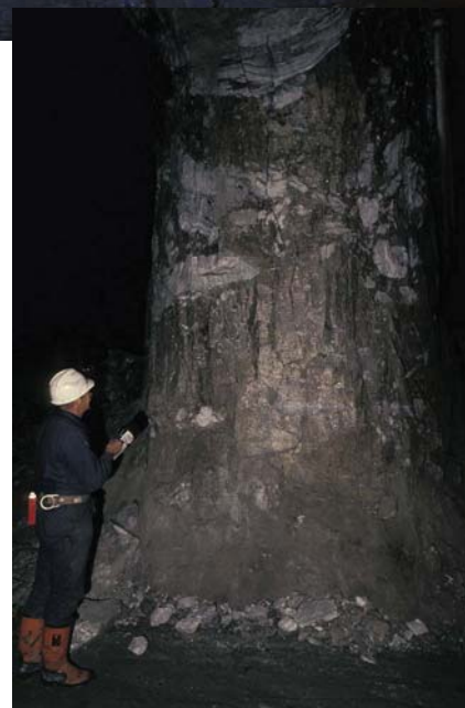
"Buck shot ore" with marble rafts left in pillar.
