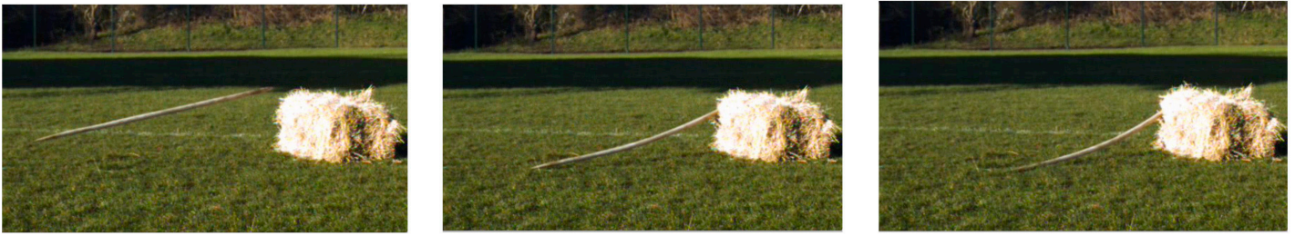
Figure 6. Sequence of three still shots from high speed video footage of a failed spear impact during a throwing experiment. The final frame demonstrates the bending of the spear when it experiences impact at both ends simultaneously, and thus the importance of the resistance of wood to rupture during throwing.
