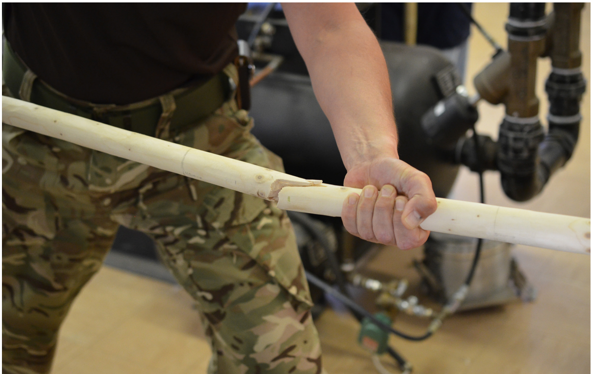
Figure 4. Example of a spear shaft breaking between the two hands during experimental use as a thrusting spear on ballistics gelatine (Milks et al. 2016). This spear shaft broke after 22 thrusts, at a point where several knots converged in the wood, representing a weak area in the wood.
