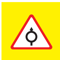
2. Roundabout straight ahead on both sides
