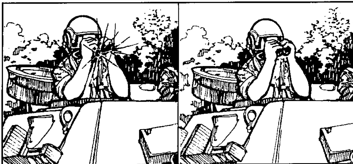
Figure E-1. Shade optics to prevent shine.
