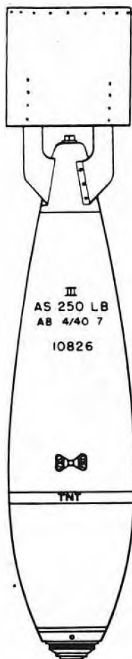
Figure 1—Typical bomb markings
