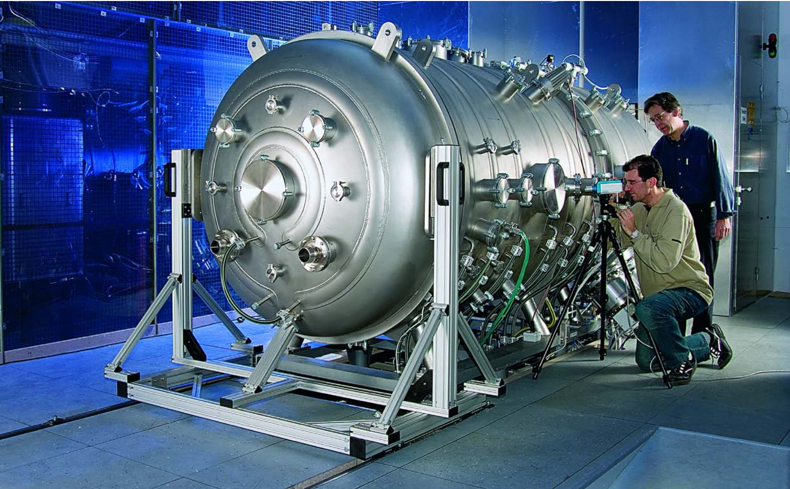
Abb. 29: Der Wärmeteststand GLADIS (Garching Large Divertor Sample Test Facility) (Foto: IPP)
