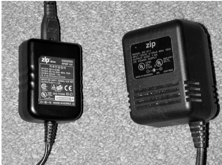
Figure 1 – Switch Mode and Linear External Power Supplies
