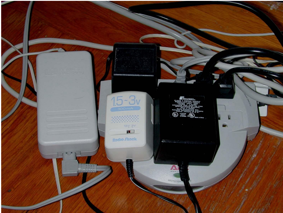
Figure 8 – The Real Reason External Power Supplies Are Known as “Wall Warts”
