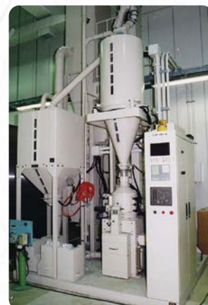
Automated rice-polishing machine. The experience of sake brewers was converted to computerized data to control this machine.
