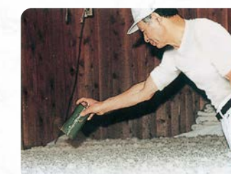
The toji (the chief sake maker) scatters koji spores onto rice in a koji -making room at a temperature approximately 30°C.
