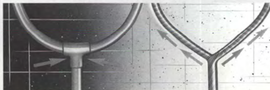
T-joints experience excessive torque at the center. The Y-joint evenly distributes the flex for more power and consistency.
