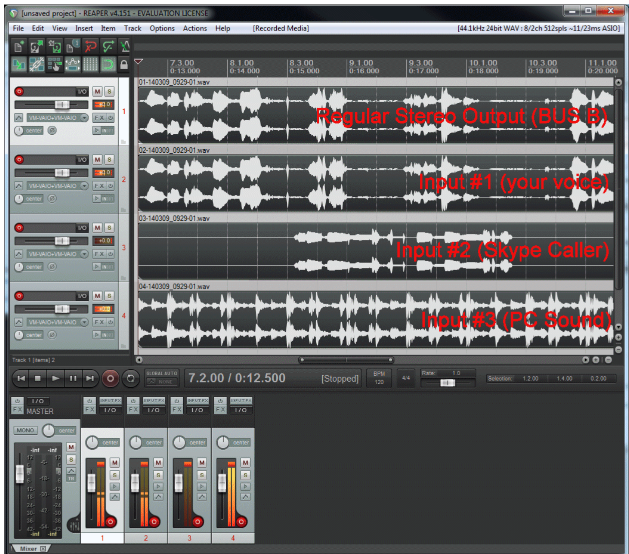
REAPER recording 4 stereo tracks coming from Voicemeeter virtual ASIO output.
